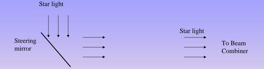
Star light is delivered to beam combiner by steering mirror.
