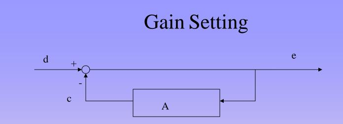
Suppose amplifier gain is adjustable.
