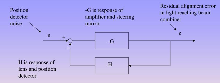
•Use –G to denote gain of amplifier because we know there is an inversion in the loop, and we like to keep the values of the gains positive
