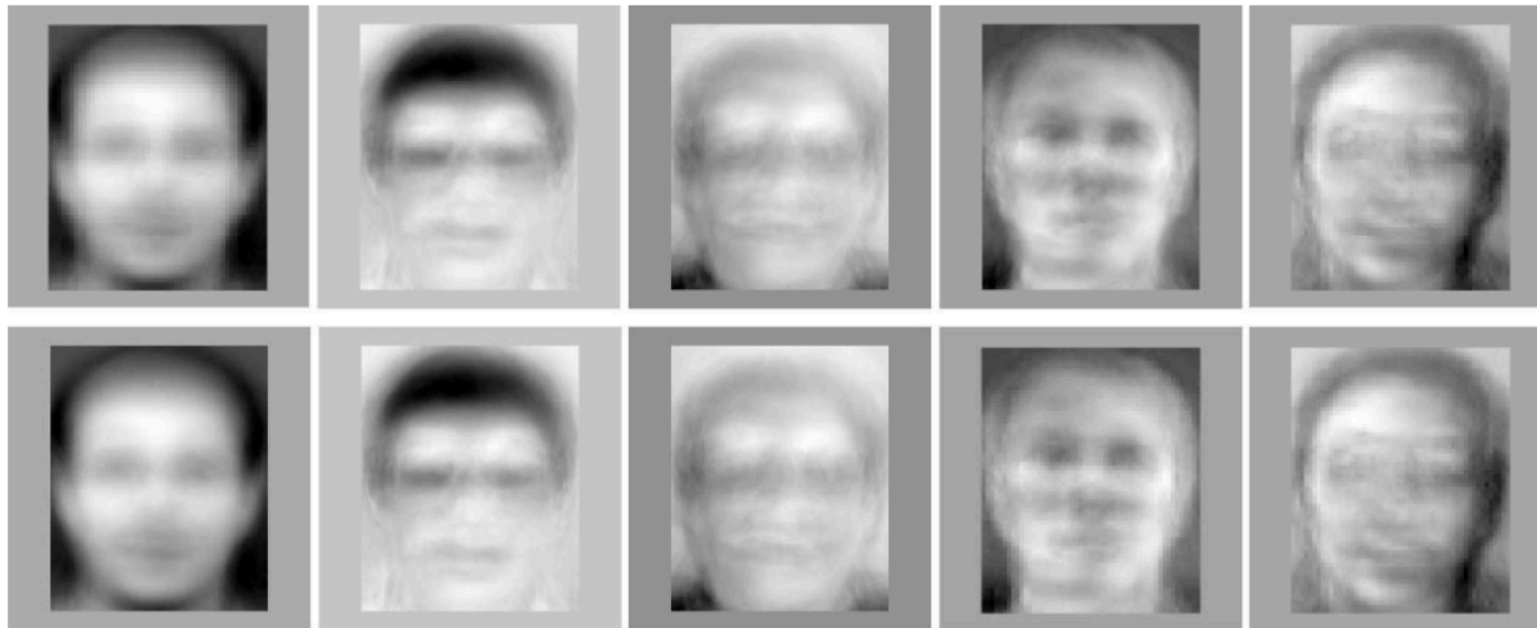
Fig. 1. The first five vectors of the KL basis (eigen-faces) produced by the standard KL algorithm (top) and the corresponding vectors produced by the proposed SKL. Scale inversion was done for some gray images to make the similarity clearer.
