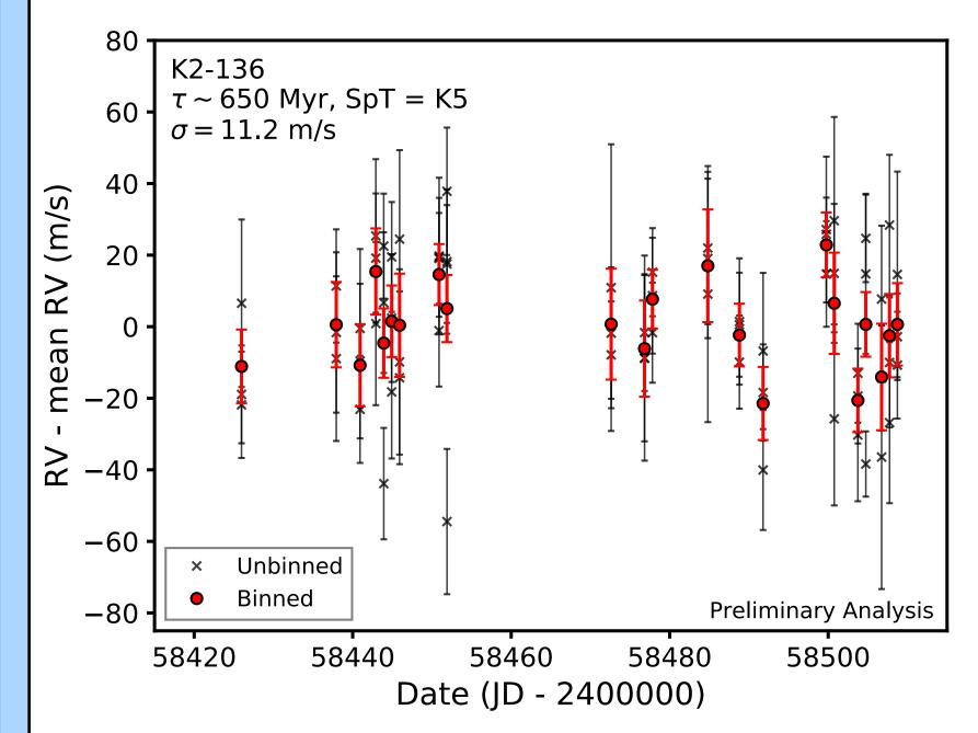
Preliminary RV time series of Hyades member K2-136 (~650 Myr, SpT=K5, Mann+ 18), with an RV precision of ~10 m/s. K2-136 demonstrates the precision achievable by our survey, as its known transiting planets' RV signals are expected to be much smaller than the stellar jitter. A 10 m/s semi-amplitude corresponds to planet masses of 25, 40, 90 M<sub>±</sub> for periods of 1 week, 1 month, and 1 year.
